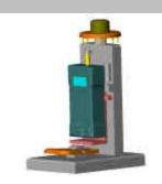
**Test station:** A test station was needed to index a lead frame an exact step, and hold it in position during a test routine. Contacts were needed to apply power to the DUT and to signal the tester to begin.
